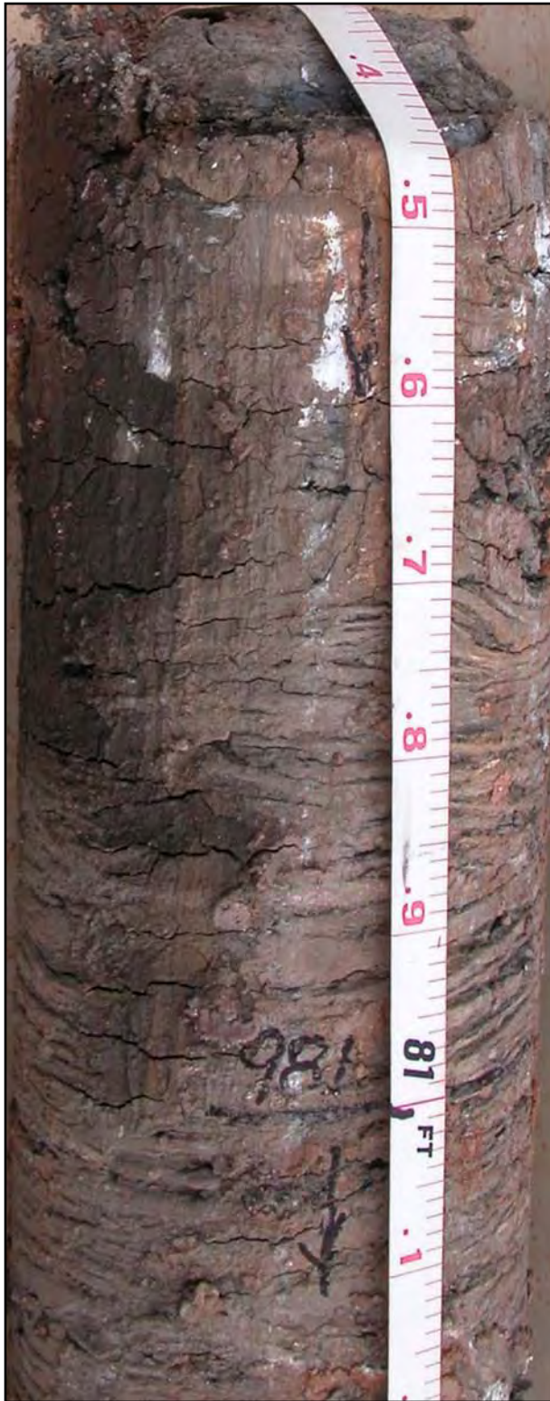
Figure 2-4. Laminar silty claystone at top of M-2 in SNL-8. Depth marking at 981.0 ft.
