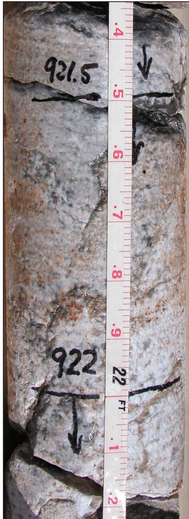
Figure 2-6. Fracturing with block rotation in lower A-3 at SNL-8. Core depth marking is 922 ft.
