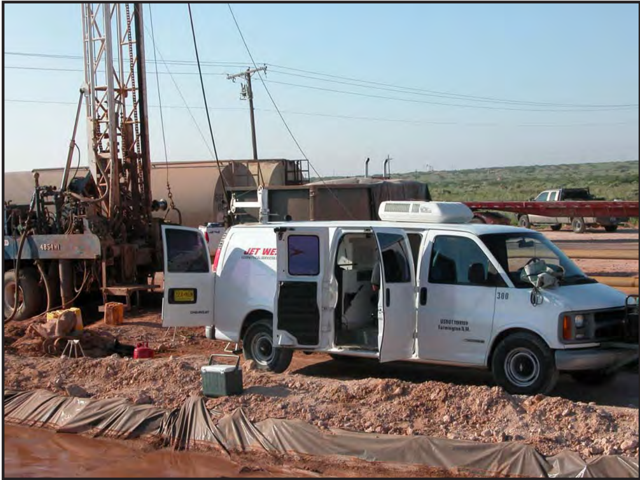
Geophysical logging at SNL-8 on June 28, 2005, by Jet West, with logging truck in position (above). Geophysical tool inside casing (right) being set with respect to the top of the surface casing before logging.
