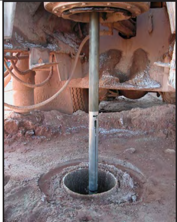
Geophysical logging at SNL-8 on June 28, 2005, by Jet West, with logging truck in position (above). Geophysical tool inside casing (right) being set with respect to the top of the surface casing before logging.
